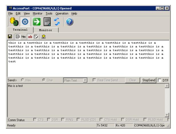
You have now made a loop-back test and confirmed that the drivers and adapter is working properly.
