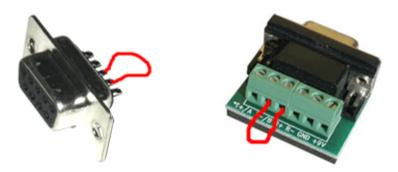
If you do not have any of these available you can manually make a connection from pin 2 to pin 3 at the adapter's DB9 connector by carefully using a piece of wire or even a paper clip to short the pins. Be careful not to short any other pins since this might damage the adapter.
