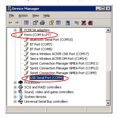
If the COM port is not listed in the Device Manager it has not been successfully created and you need to determine the cause. This could be due to incorrect drivers, conflicting drivers if you have other USB serial drivers installed, or simply an unsuccessful driver installation. A solution could be to uninstall all current USB serial drivers, reboot and re-install the most recent drivers again. Notice: a reboot is highly recommended after each driver un-installation/installation.
