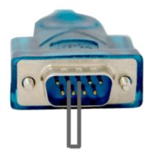
With the COM port open in AccessPort and the TX / RX pins connected together the text string should now be sent out through the TX pin, looped back through the RX pin and received in the 'receive' window:
