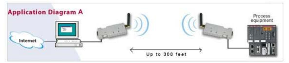
One to one communication between a computer and a serial device or between two serial devices. This is often used if the computer has no built-in Bluetooth or if you need an easy to setup cable replacement.
