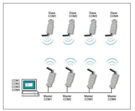
Multiple pairs serial Bluetooth adapters. Ideal for applications where multiple links in pairs are needed, (max 255).
