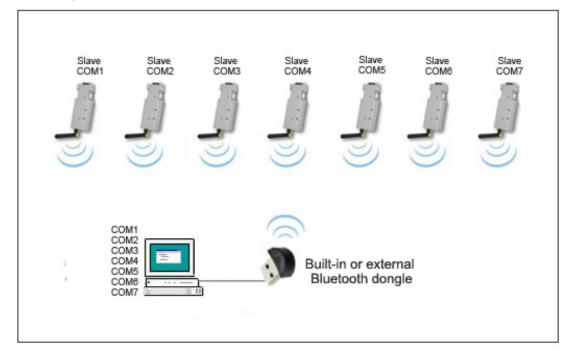
Ideal for applications where multiple links are needed, (max 255). Multiple COM ports are created at the local computer. Each COM port will show up in your computer's COM port and can be used as if it was a built-in COM port.
