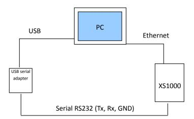
TX, RX and GND must be properly connected between the XS1000 and the USB serial adapter
