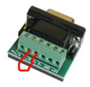
If you do not have any of these available you can manually make a connection from pin 2 to pin 3 at the DB9 connector by carefully using a piece of wire or even a paper clip to short the pins, as shown in the image below. Be careful not to short any other pins since this might damage the adapter.
