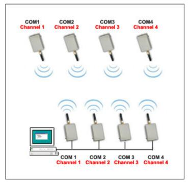
Point-to-multipoint configuration, multiple masters with different channels and different COM ports
