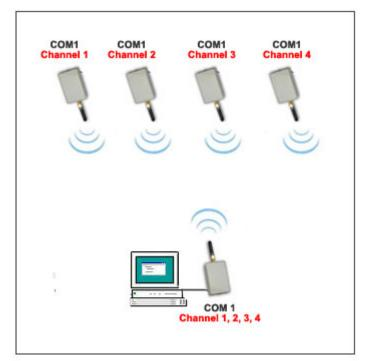
Point-to-multipoint configuration, one master with different slave channels and different COM ports.
